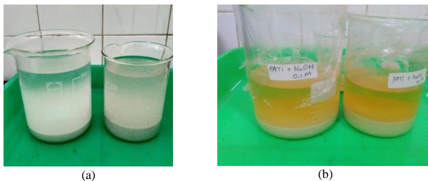
Figure 1. Washing process of arrowroot starch by (a) water and (b) 0.1 M NaOH
