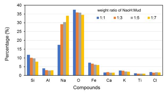
Figure 2. Composition of elements in the smelting sample at various weight ratios of NaOH/mud from XRF analysis
