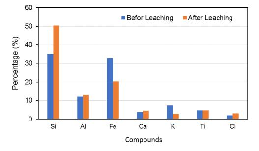
Figure 1. The composition of the sludge from the XRF analysis before and after the leaching process
