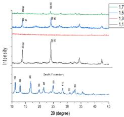
Figure 3. Standard Zeolite Y Diffractogram and Zeolite Y Diffractogram Synthesis Results Variation of NaOH/mud weight ratio
