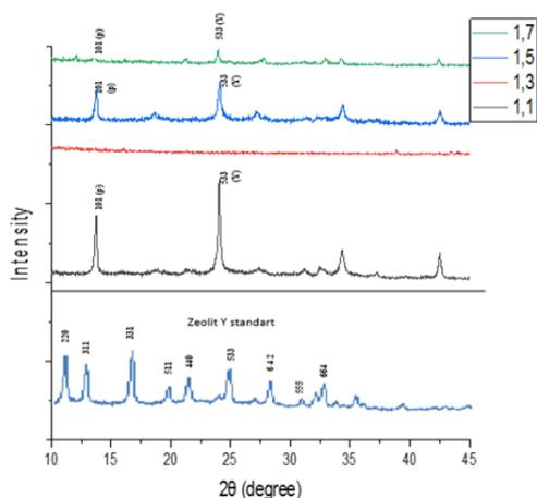
Figure 3. Standard Zeolite Y Diffractogram and Zeolite Y Diffractogram Synthesis Results Variation of NaOH/mud weight ratio
