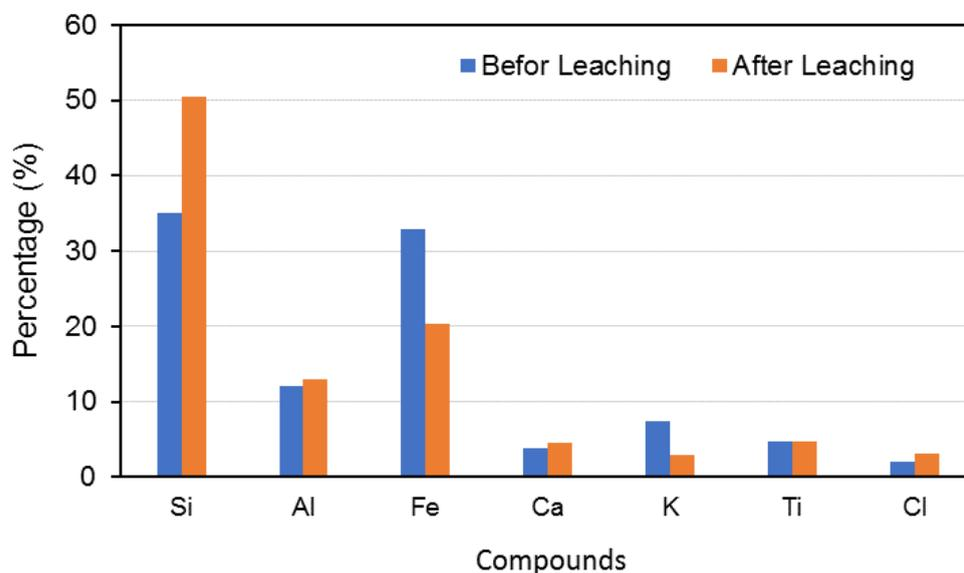
Figure 1. The composition of the sludge from the XRF analysis before and after the leaching process
