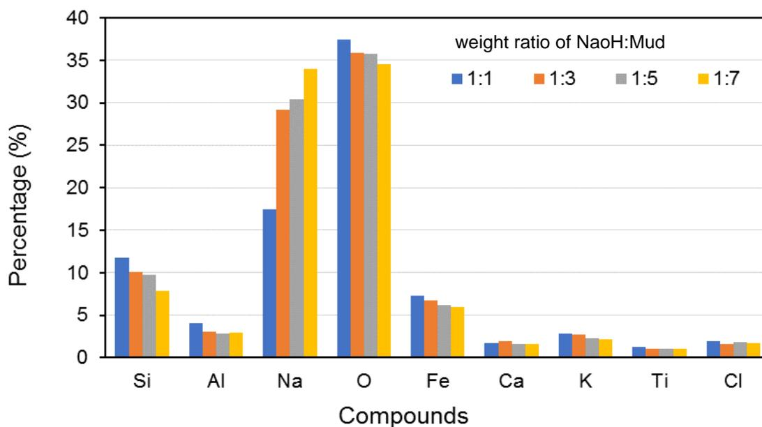
Figure 2. Composition of elements in the smelting sample at various weight ratios of NaOH/mud from XRF analysis
