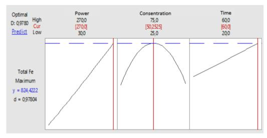
Figure 4. Graph of optimization plot with the UAE method
