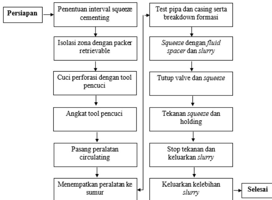
Gambar 3.1 Prosedur Squeeze Cementing
